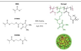
Scheme 1 Synthesis of DTM-labelled nanogels by radical cross-linking emulsion polymerisation.
