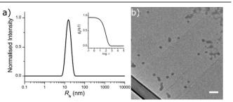
**Fig. 1** a) Size distribution obtained by DLS (detection angle of 90°) for a solution of **NG2** at 1 g/L, and the corresponding autocorrelation function (inset); b) **NG2** imaged by TEM on a GO support. The particles showed a tendency to aggregate upon drying (top right corner). Scale bar 100 nm
