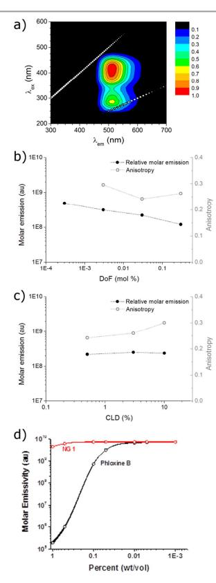
**Fig. 2** a) 2D excitation-emission spectra with a 5 nm step for aqueous solution of **NG1**. b) Molar emission and anisotropy for nanogels with CLD = 0.5 wt% with variable *DoF* (**NG1,2,5,6**), and c) *DoF* = 0.03 mol% with variable *CLD* (**NG2-4**). d) Molar emissivity *vs* concentration for aqueous solutions of **NG1** and Phloxine B
