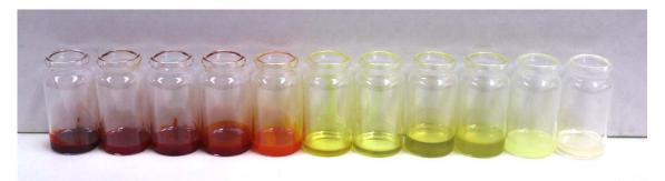
**Figure 1.**  $[C_4C_1Im]^+$  based halobismuthate ionic liquids with different anions (from left to right):  $[Bil_3Br]^-$ ,  $[Bil_3Cl]^-$ ,  $[BiBr_2l_2]^-$ ,  $[BiCl_2l_2]^-$ ,  $[BiBr_2Cl1]^-$ ,  $[BiBr_3Cl]^-$ ,  $[BiBr_3Cl]^-$ ,  $[BiBr_3Cl]^-$ ,  $[BiBr_2Cl_2]^-$ ,  $[BiBr_2Cl_2]^-$ ,  $[BiBrCl_3]^-$ ,  $[BiCl_4]^-$ .
