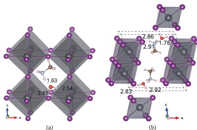
Fig. 1 Polyhedral view of water intercalated phase MAPbI<sub>3</sub>·H<sub>2</sub>O (a) and monohydrated phase MAPbI<sub>3</sub>·H<sub>2</sub>O (b). Hydrogen bonds are marked with dotted lines and the bond lengths are presented in units of angstrom (dark grey: Pb; purple: I; brown: C; light blue: N; red: O; light pink: H).
