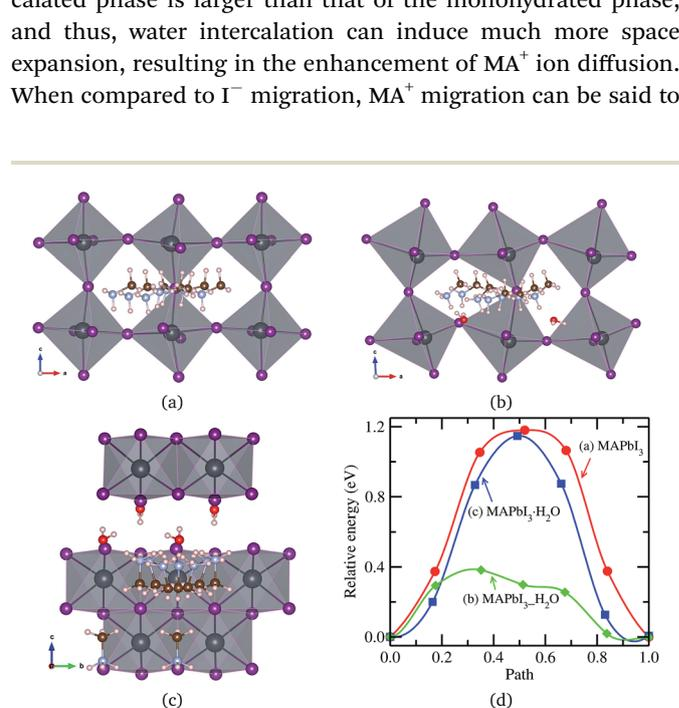
Fig. 5 MA<sup>+</sup> ion migration in (a) pseudo-cubic MAPbI<sub>3</sub>, (b) water intercalated phase MAPbI<sub>3</sub>·H<sub>2</sub>O and (c) monohydrated phase MAPbI<sub>3</sub>·H<sub>2</sub>O, and (d) corresponding activation energy profile.
