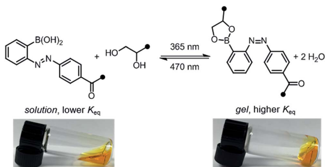
Fig. 4 Reversible sol–gel transition of a mixture of P1 and P2 (1 : 1, 10 w/v% in PBS, pH 7.5). Gelation was performed by irradiation with 365 nm light (10 min, 3.6 mW cm −2 ); gelation was reversed by irradiation with 470 nm light (30 s, 900 lux).
