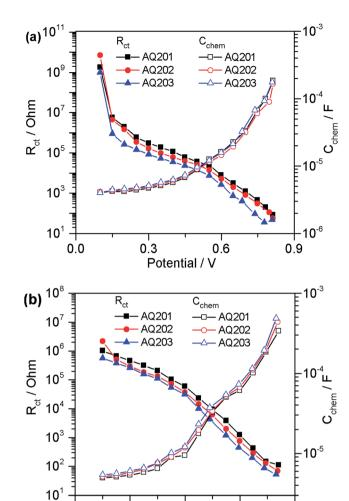
Fig. 5 Charge transfer resistance ( $R_{\rm ct}$ ) and chemical capacitance ( $C_{\rm chem}$ ) plotted against the IR drop corrected potential for DSSCs based on dyes AQ201, AQ202, and AQ203 with (a) the [Co(bpy)<sub>3</sub>]<sup>2+/3+</sup> redox electrolyte and (b) the I<sup>-</sup>/I<sub>3</sub><sup>-</sup> redox electrolyte.
