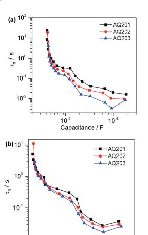
Fig. 6 Electron lifetime  $(\tau_n)$  plotted against chemical capacitance  $(C_{\text{chem}})$  of DSSCs based on dyes AQ201, AQ202, and AQ203 with (a) the  $[\text{Co(bpy)}_3]^{2+/3+}$  redox electrolyte and (b) the  $I^-/I_3^-$  redox electrolyte.
