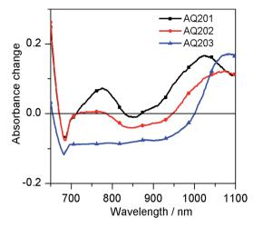
Fig. 7 PIA spectra measured upon laser excitation ( $\lambda_{exc}=510$  nm) of AQ201, AQ202 and AQ203 dyes adsorbed on 4  $\mu$ m mesoporous TiO<sub>2</sub> films in the absence of redox electrolytes.
