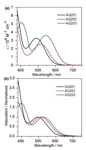
Fig. 1 (a) Absorption spectra of dyes AQ201, AQ202, and AQ203 in CH<sub>2</sub>Cl<sub>2</sub>; (b) normalized absorption spectra of dyes AQ201, AQ202, and AQ203 on 4 µm TiO2 films
