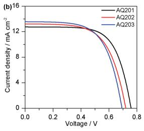
Fig. 3 J-V curves of DSSCs based on dyes AQ201, AQ202, and AQ203 with (a) the  $[Co(bpy)_3]^{2+/3+}$  redox electrolyte and (b) the I<sup>-</sup>/I<sub>3</sub><sup>-</sup>redox electrolyte.
