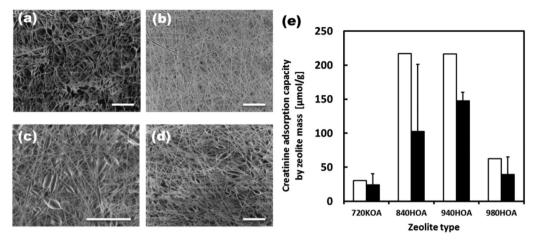
Fig. 5 SEM images of zeolite–EVOH nanofiber composites with various types of zeolites (10 wt%). (a) 720-KOA (Ferrite), (b) 840-HOA (ZSM-5), (c) 940-HOA (beta), and (d) 980-HOA (beta) (scale bar: 20  $\mu$ m). (e) Creatinine adsorption capacities of free zeolites (open) and those in the fiber by zeolite mass (closed) after 24 h of immersion (n = 3).
