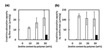
Fig. 6 Creatinine adsorption capacity of 940-HOA zeolite nanofibers by fiber mass (a) and zeolite mass (b) in the absence (open bar) or presence (closed bar) of flow (n = 3). The absorption capacities were obtained after 24 h or 5 h for batch (no flow) or circulating (under flow) experiments, respectively.
