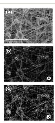
Fig. 3 SEM/EDX mapping images of beta-type 940-HOA zeolite (10 wt%)–EVOH nanofiber composite produced from 7 w/v% HFIP (scale bar: 8  $\mu$ m). (a) SEM, (b) O-mapping, and (c) Si-mapping.
