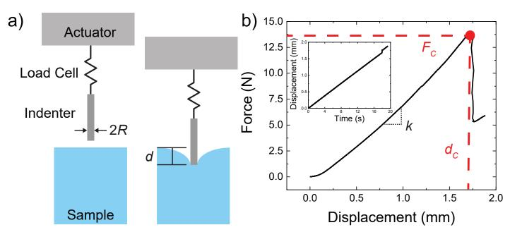
Fig. 2 a) Sketch of the deep indentation and puncture measurements. b) Plot of the force displacement curve with the critical puncture force and displacement marked in red. The inset graph shows the displacement vs time profile.
