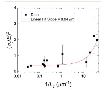
**Fig. 5** Plot showing  $(\sigma_c/E)^2$  against  $1/L_c$  for the composite hydrogels used in this study. Note that the x-axis is plotted in log scale. The slope on this plot, 0.04  $\mu$ m, is well below the elastofracture length of these materials and no significant transition is observed. This likely indicates that the assumption that  $a=L_c$  in the absence of a macroscopic notch is incorrect.
