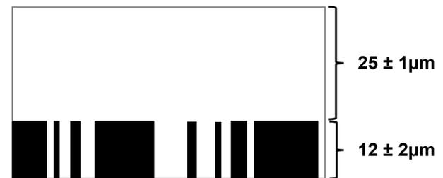
Fig. 2 Top: The sandstone-like pattern printed and etched on the wafer to create the fracture roughness. The x-length of the pattern is 350  $\mu\text{m}$ . Bottom: The topography of the etching of the fracture aperture and the side view of the fracture roughness.
