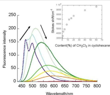
**Fig. 7** Fluorescence spectra of **11** in mixed solvents of  $\text{CH}_2\text{Cl}_2$ - $\text{C}_6\text{H}_{12}$ .  $\text{CH}_2\text{Cl}_2$  content: 0% (dark blue), 1% (blue), 4% (light blue), 8% (green), 12% (yellowish green), 16% (yellow), 20% (orange), 40% (red) and 60% (dark red). Reproduced from Ref.<sup>71</sup>
