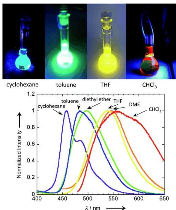
Fig. 14 Fluorescence color (photographs) and normalized fluorescence spectra of **24** in various solvents. Copyright 2021 Wiley. Used with permission from Ref. <sup>85</sup>
