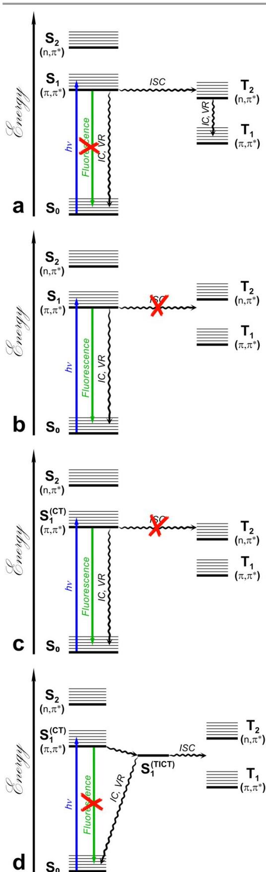
**Fig. 34** Jablonski diagrams illustrating possible deactivation pathways of photoexcited nitroaromatic chromophores. (ISC = intersystem crossing, IC = internal conversion, and VR = vibrational relaxation)
