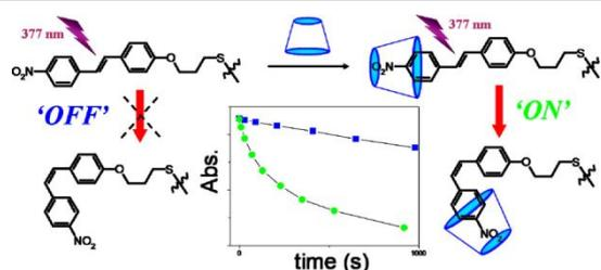
**Fig. 4** A host-guest complex with  $\beta$ -cyclodextrin ( $\beta$ -CD) diminishes H-bonding, resulting in both a blue-shift of the fluorescence maximum along with an increase in the fluorescence response. Reprinted with permission from Ref. <sup>69</sup> Copyright 2012 American Chemical Society.
