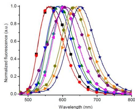
Fig. 21 Normalized fluorescence of **48** in toluene (■), diethyl ether (●), THF (▲), ethyl acetate (▼), CHCl<sub>3</sub> (◆), CH<sub>2</sub>Cl<sub>2</sub> (◄), DMF (►) CH<sub>3</sub>CN (●), DMSO (★) and ethanol (◆). Reproduced from Ref.<sup>102</sup>
