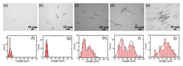
Fig. 2 (a)-(e) Optical micrographs of the microrods after growing for 12 (a), 19 (b), 39 (c), 55 (d) and 82 (e) days, respectively. (f) - (j) The corresponding histograms of the microrod lengths. Curves are Gaussian fits to the histograms.
