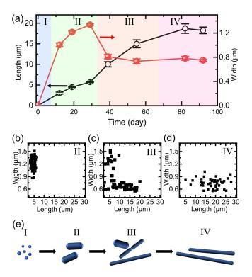
Fig. 3 (a) The time-dependent lengths (black circles) and widths (red dots) of the microrods. (b) - (d) The morphology of the microrods in growth stages of II (b), III (c) and IV (d) represented by plotting their lengths versus widths. (e) A sketch of the microrod growth process.
