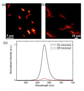
**Fig. 4** (a), (b) Scanning photoluminescence images of short (a) and long (b) microrods from two different growth stages spin coated with quantum dots. (c) Photoluminescence spectra taken from the microrods and from the adjacent background area.
