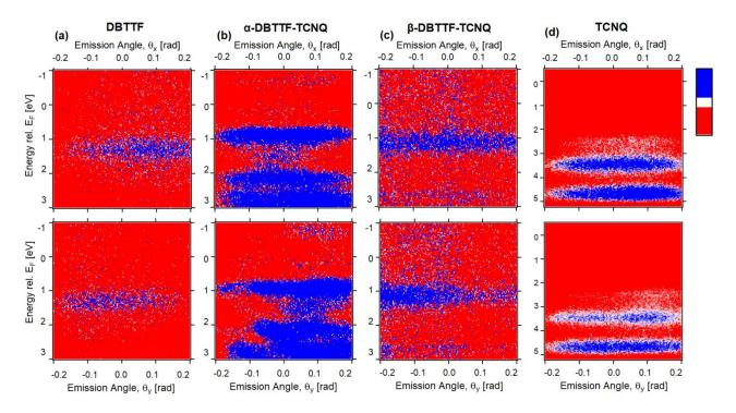
Figure 3. ARPES results of crystalline (a) DBTTF, (b)  $\alpha$ -DBTTF-TCNQ, (c)  $\beta$ -DBTTF-TCNQ, and (d) TCNQ. Top and bottom panel show the electron emission as a function of  $\theta_x$  and  $\theta_y$ , respectively, and high counts shown in blue and low counts in red. The data are shown within the angular emission range of  $\pm$  0.2 rad (corresponding to  $\pm$  0.8 Å<sup>-1</sup>).
