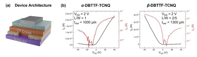
Figure 2: a) the bottom-contact, top-gate transistor architecture used to extract the trap-DOS for each polymorph. b) Examples of transfer characteristics in the linear regime for each polymorph. The  $V_{DS}$ , channel dimensions as a ratio of length to width (L/W), and thickness of the parylene-N gate dielectric ( $t_{Pary}$ ) are given in the inset.
