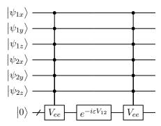
**Fig. 2** Canonical quantum circuit to implement  $\exp(-i arepsilon \hat{V}_{ee}) \ket{\psi_{12}}$  on a quantum computer. The function evaluation,  $V_{12} = V_{ee}(x_1, y_1, z_1, x_2, y_2, z_2)$ , involves six explicit coordinates and sets of qubits, and includes an inverse square-root evaluation.
