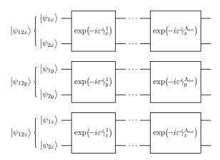
**Fig. 4** CCS quantum circuit to implement  $\exp(-i\epsilon\hat{V}_{ee}) |\psi_{12}\rangle$  on a quantum computer, based on Eq. (9). The six-dimensional  $V_{ee}$  function gate of Fig. 2 is now replaced with two-dimensional function gates, which separate by Cartesian component. The two-particle wavefunction contribution  $|\psi_{12}\rangle$  decomposes naturally into  $|\psi_{12x}\rangle$ ,  $|\psi_{12y}\rangle$ , and  $|\psi_{12z}\rangle$  components.
