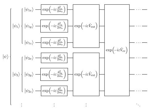
Fig. 1 Overview of quantum circuit to implement unitary short time evolution,  $\hat{U}(\varepsilon)|\psi\rangle$ , via Trotterization, on a quantum computer. This structure is used in both the canonical and CCS Trotter quantum circuitry.
