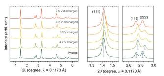
Fig. 4 Synchrotron XRD patterns of LT-Li $Mn_{0.5}Ni_{0.5}O_2$  electrodes at various states of charge (1<sup>st</sup> cycle).
