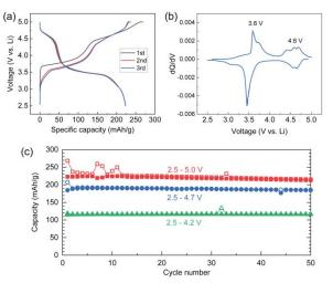
**Fig. 3** (a) Voltage profiles of Li/LT-LiMn<sub>0.5</sub>Ni<sub>0.5</sub>O<sub>2</sub> cells (i = 15 mA/g), (b) corresponding differential capacity (dQ/dV) plot (2nd cycle), and (c) cycling stability (open = charge, solid = discharge).
