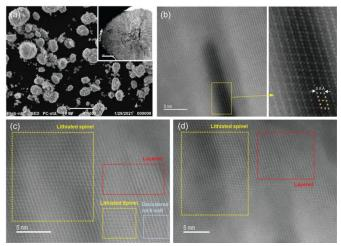
Fig. 2 (a) SEM and (b-d) HAADF-STEM images of LT-LiMn $_{0.5}Ni_{0.5}O_2$ .
