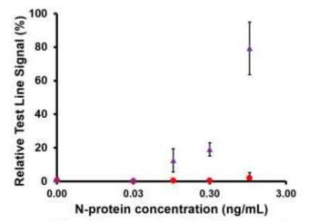
Fig. 7 Plot of relative test line signal intensity versus N-protein concentration for both the LFA (red  $\bullet$ ) and enhancement steps (purple  $\blacktriangle$ ). Data is represented as the mean  $\pm$  SD (n = 4).
