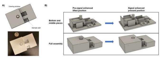
Fig. 4 (A) CAD drawing (top) and 3D printed (bottom) full casing assembly with labelled viewing window and sample well. US quarter included for size comparison. (B) CAD drawings showing the casing before and after pressing the middle piece.
