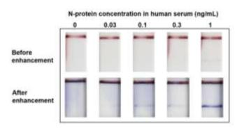
**Fig. 6** Detection of the N-protein of SARS-CoV-2 in human serum using nanozyme signal enhanced LFA. Detection limit before enhancement is 1 ng/mL while after enhancement it is 0.1 ng/mL, demonstrating at least a 10-fold improvement in detection limit and detection of N-protein within the desired concentration range.
