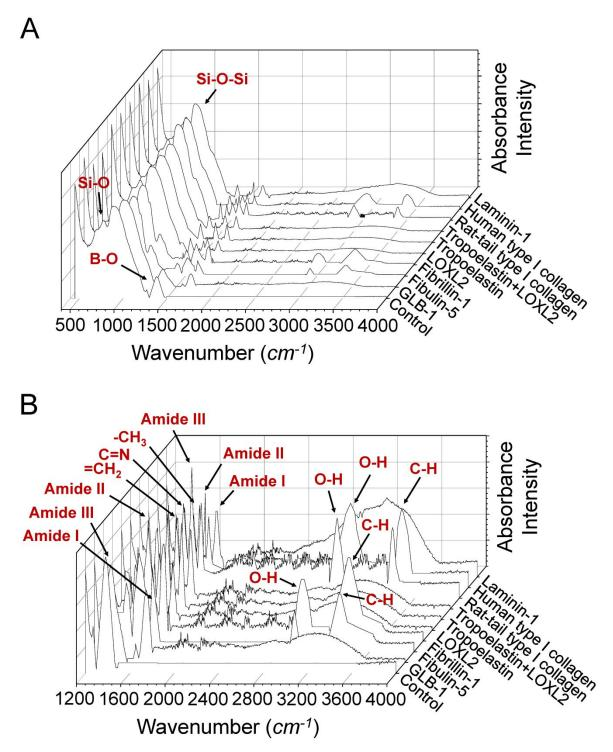
**Figure 2.** FTIR absorption intensities in (A)  $500 - 4000 \ cm^{-1}$  and (B)  $1200 - 4000 \ cm^{-1}$  range obtained using a Spectrum Two FT-IR Spectrometer. All samples show characteristic absorption peaks at ~1000  $\ cm^{-1}$  and ~850  $\ cm^{-1}$  which represent the silicon-oxygen-silicon stretching and silicon-oxygen peaks inherent of the non-coated borosilicate cover glass.
