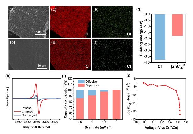
**Fig. 5** The SEM images of CLPy at cathode (a) charged and (b) discharged states. The elemental mapping of C at (c) charged and (d) discharged states. The elemental mapping of Cl at (e) charged and (f) discharged states. (g) The calculated binding energy of  $Cl^-$  and  $[ZnCl_4]^{2-}$  in CLPy. (h) The EPR spectra of CLPy cathode at different states. (i) The capacity composition at different scan rates. (j) The calculated diffusivity of  $Cl^-$  in CLPy cathode based on GITT.
