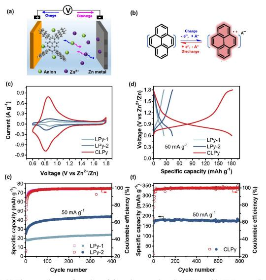
**Fig. 2** (a) The operation configuration of the polypyrene-based AZDIBs with CLPy as cathode. (b) The charge storage mechanism of polypyrene cathode. (c) The CV curves of polypyrenes at 0.5 mV s<sup>-1</sup>. (d) GCD potential curves for the three polypyrene cathodes at 50 mA g<sup>-1</sup> at the 400<sup>th</sup> cycle. The cycling performance of (e) LPy-1, LPy-2 and (f) CLPy at 50 mA g<sup>-1</sup>.
