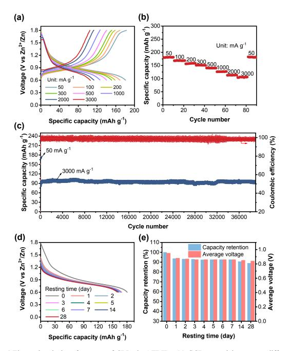
**Fig. 4** Electrochemical performance of CLPy in AZDIBs. (a) GCD potential curves at different current rates. (b) Rate performance at currents from 50 to 3000 mA  $g^{-1}$ . (c) Cycling performance at 3000 mA  $g^{-1}$ . (d) Discharge curves after resting different times. (e) The capacity retention and average voltage *vs* Zn<sup>2+</sup>/Zn after resting different times.
