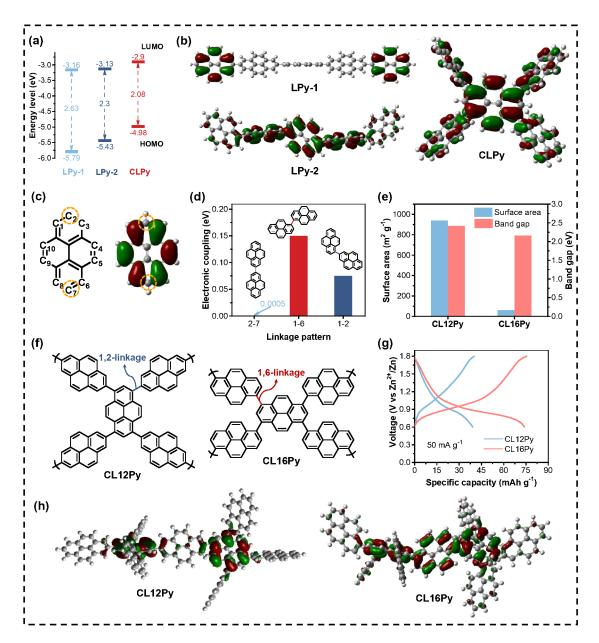
**Fig. 3** (a) The energy levels and (b) the HOMO diagram of LPy-1, LPy-2 and CLPy. (c) The structure with numbered carbon (left) and the HOMO diagram (right) for the pyrene unit. (d) The electronic coupling for different linking patterns of bipyrene. (e) The surface area and band gaps of CL12Py and CL16Py. (f) The polymer structures of CL12Py and CL16Py. (g) The GCD
