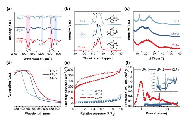
**Fig. 1** The characterization of polypyrenes. (a) The FT-IR spectra. (b) The solid-state NMR spectra. (c) The XRD patterns. (d) UV/Vis absorption spectra. (e) The  $N_2$  adsorption (filled symbols)/desorption (open symbols) isotherms. (f) The PSD curves calculated by NL-DFT (Inset: the PSD curves of LPy-1 and LPy-2).
