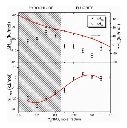
Figure 4 Enthalpies of drop solution and formation from binary oxides (top), enthalpies of mixing (bottom) of Y<sub>3</sub>NbO<sub>7</sub> - Y<sub>2</sub>Ti<sub>2</sub>O<sub>7</sub> solid solutions. The error is two standard deviations of the mean.
