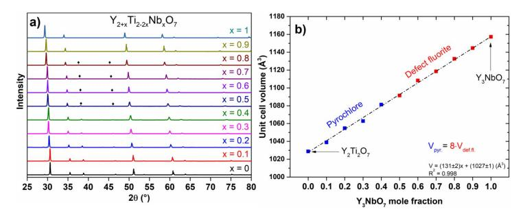
Figure 2 a) X-ray diffractograms of synthesized  $Y_{2+x}Ti_{2-2x}Nb_xO_7$  solid solutions. Black diamonds mark the reflections around 38° and 47° which correspond to additional pyrochlore ordering, b) normalized volume of the unit cell of  $Y_{2+x}Ti_{2-2x}Nb_xO_7$ .
