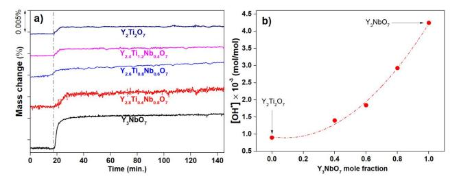
Figure 3 a) Thermograms of investigated samples under the isothermal switch between dry and wet gas. b) protonic defect concentration vs Y<sub>3</sub>NbO<sub>7</sub> mole fraction.
