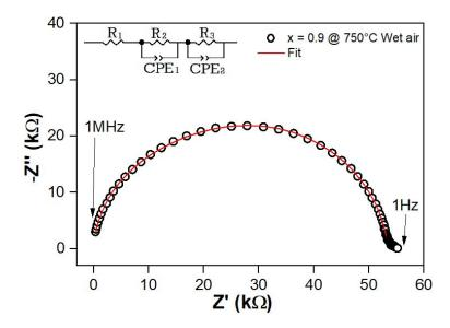
Figure 5 Typical complex impedance data (open symbols) with the fit (line) and corresponding equivalent circuit exemplified for Y<sub>2.9</sub>Ti<sub>0.2</sub>Nb<sub>0.9</sub>O<sub>7</sub>.
