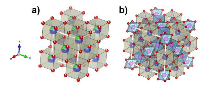
Figure 1 a)  $Y_3NbO_7$  defect fluorite structure ( $Fm\overline{3}m$ ). b)  $Y_2Ti_2O_7$  pyrochlore structure ( $Fd\overline{3}m$ ). Colors: blue – yttrium, green – niobium, red – oxygen, white – oxygen vacancies, purple – titanium. Unit cell edges are marked with thick white lines. Pictures prepared by Vesta Software<sup>13</sup>.
