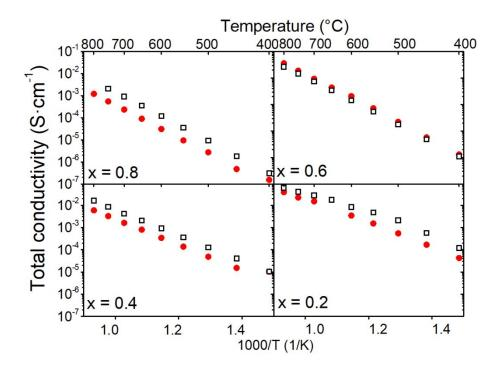
Figure 8 Total conductivity as a function of inverse temperature for Y<sub>2+x</sub>Ti<sub>2-2x</sub>Nb<sub>x</sub>O<sub>7</sub> samples, collected in dry hydrogen (open squares) and wet hydrogen (red circles)
