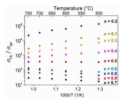
Figure 9 Temperature dependence of the ratio of conductivity in dry hydrogen and dry air for the solid solutions with different Y<sub>3</sub>NbO<sub>7</sub> mole fractions (x).
