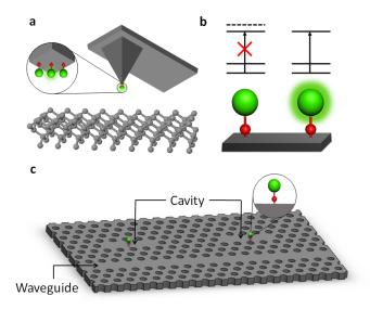
**Figure 6**. Applications of surface bound OCCs. (a) An AFM/STM tip can be functionalized with OCC centers, enabling precision quantum-enhance readout of local magnetic and electric fields through fluorescence. (b) Two OCCs in spatial proximity can provide the two qubit basis for a CNOT gate achieved through dipole blockade. (c) OCCs can be placed in a photonic waveguide, entangling two OCCs via photonic bus.
