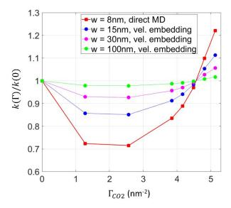
Fig. 2. Variation of the decane permeability of calcite slit pores at different CO<sub>2</sub> adsorption densities  $\Gamma_{co2}$ .
