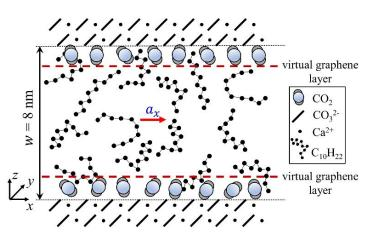
Fig. 1. A schematic of the simulation system for studying decane transport through slit calcite pores. Virtual graphene layers (red dashed lines) interacting only with  $CO_2$  confine them near the calcite surface to ensure a well-defined  $CO_2$  adsorption density during simulation. z = 0 corresponds to the uppermost oxygen atom layer of the lower calcite slab.
