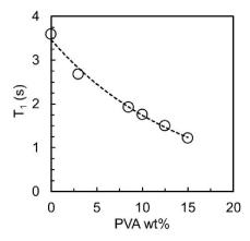
**Figure 3**.  $^{7}$ Li spin-lattice relaxation time ( $T_{1}$ ) as a function of PVA3 concentration in LNH measured at 22 °C.
