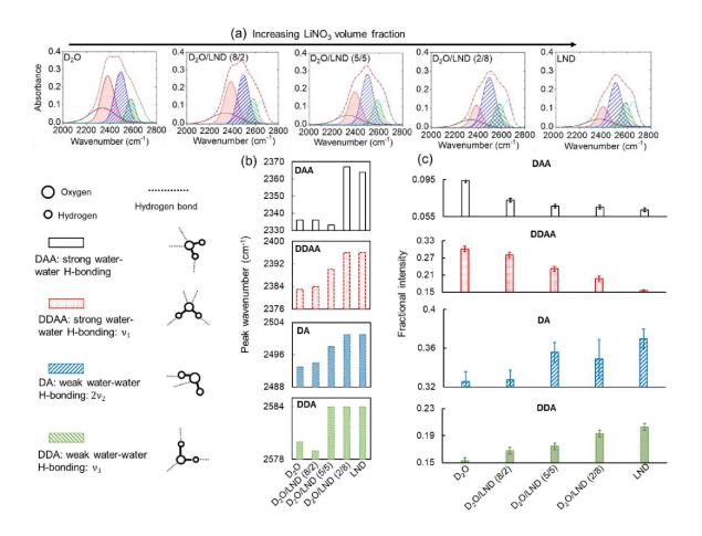
**Figure 2**. FTIR analysis of 2000-2800 cm-1 –OD vibrational region in LND, D2O, and D2O/LND mixed solvents (a), peak wavenumber (b) and fractional intensity (c) changes corresponding to the deconvoluted peaks of DAA, DDAA, DA, and DDA vibrations upon gradual transition from D2O to LND.
