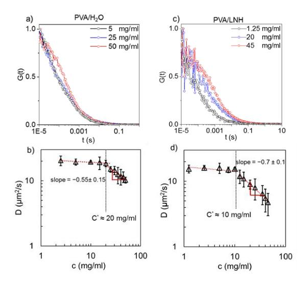
Figure 5. FCS autocorrelation functions and diffusion coefficients in  $10^{-4}$  mg/ml PVA2\* solutions in water (a,b) and LNH (c, d), which also contained increasing amounts of unlabeled PVA2 with  $M_w$  of 69,000 g/mol. Temperature was 22 °C.
