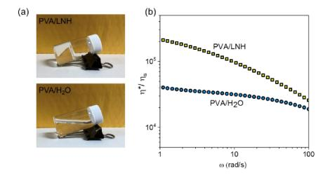
**Figure 1**. Digital images (a) and frequency dependence of the relative shear viscosities (b) of 15% PVA3 solutions in LNH and water at T = 22 °C.
