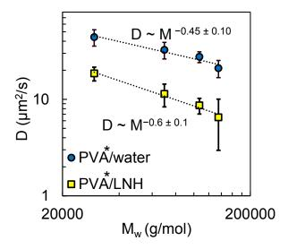
**Figure 4**. Molecular weight dependences of FCS diffusion coefficients of PVA\* measured in 10<sup>-4</sup> mg/ml aqueous or LNH solutions at 22 °C.
