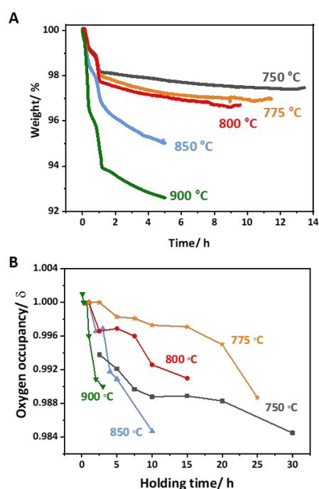
**Figure 4.** Lithium and oxygen loss in NMC71515 during sintering. (A) Weight loss of NMC71515 during holding at different temperatures, measured by TGA. The samples were heated at a rate of 5 K s<sup>-1</sup>. (B) Oxygen occupancy ( $\text{O}_{\text{6c}}$ ) as a function of holding time at different temperatures.
