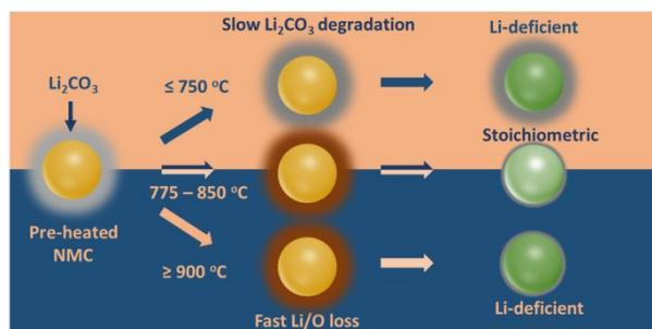
Surface reconstruction reactions that would determine the Li/Ni ordering in Ni-rich layered materials are investigated.
