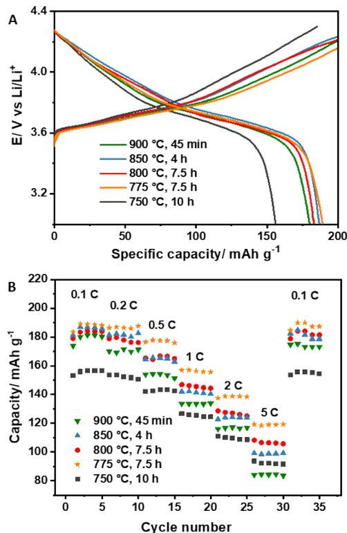
**Figure 5.** Electrochemical performance of NMC71515 sintered at different temperatures. (A) Galvanostatic charge/discharge profiles and (B) rate performances of NMC 71515 sintered for optimized time ( $t_0$ ) at different temperatures (1 C = 200  $\text{mA g}^{-1}$ ). The areal loading of active material is approximately  $0.8 \text{ mg cm}^{-2}$ .
