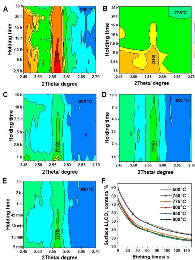
**Figure 3.** Formation of  $\text{Li}_2\text{CO}_3$  with holding time at different temperatures. (A-E) Contour plots of the XRD patterns in the selected  $2\theta$  regions containing  $\text{Li}_2\text{CO}_3$  (110) peak at sintering temperatures from 750 °C to 900 °C. (F)  $\text{Li}_2\text{CO}_3$  contents measured from XPS for different etching time (estimated from the ratio of peak areas for  $\text{O}_{\text{Li}_2\text{CO}_3}:\text{O}_{\text{Total}}$ ).
