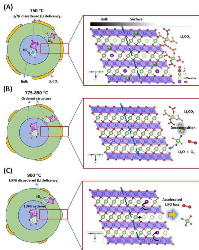
**Scheme 1.** Schematic illustrations of how cationic ordering is coupled to surface reconstruction of NMC71515 under different sintering temperatures: (A) when the temperature is too low, unreacted  $\text{Li}_2\text{CO}_3$  leads to Li-deficient phase in the bulk; (B) under ideal sintering condition, a Li/Ni ordered structure can be achieved due to the decomposition of  $\text{Li}_2\text{CO}_3$ ; (C) when the temperature is too high, Li/O loss from the surface brings about Li-deficient phase.
