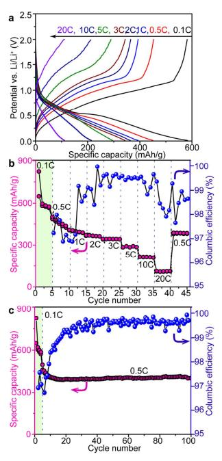
**Fig. 3** The rate performance of the  $Ni_5P_4$ : a) discharge-charge profiles at different cycling rates. b) the specific capacity as a function of rate, and c) the high-rate performance over extended cycling.
