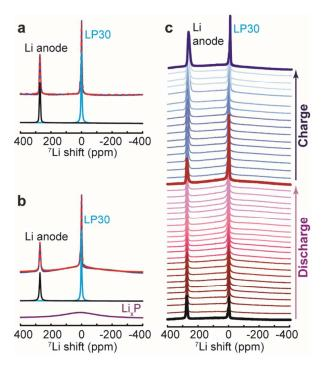
**Fig. 6** <sup>7</sup>Li NMR spectra and the corresponding spectral simulation for a pristine (a) and a fully discharged (b)
