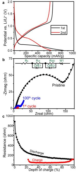
**Fig. 2** Electrochemical performance of the  $Ni_5P_4$  anode in  $Ni_5P_4/Li$  half cells. a) discharge-charge profile for the first 2 cycles, b) Electrochemical Impedance Spectroscopy (EIS) spectra of a pristine  $Ni_5P_4/Li$  battery, and the same battery after the 1<sup>st</sup> and 100<sup>th</sup> discharge-charge cycles, and c) DC resistance at different depths of charge during the first discharge-charge cycle, obtained from GITT measurements (Fig. S6).
