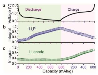
**Fig. 7** a) Electrochemical profile of a Ni<sub>5</sub>P<sub>4</sub>//Li half-cell battery in the working voltage window between 2.0 and 0.0 V. b) and c) Normalized area integrals of the  $Li_xP$  and Li resonances from *in operando* <sup>7</sup>Li NMR shown in Fig. 6.
