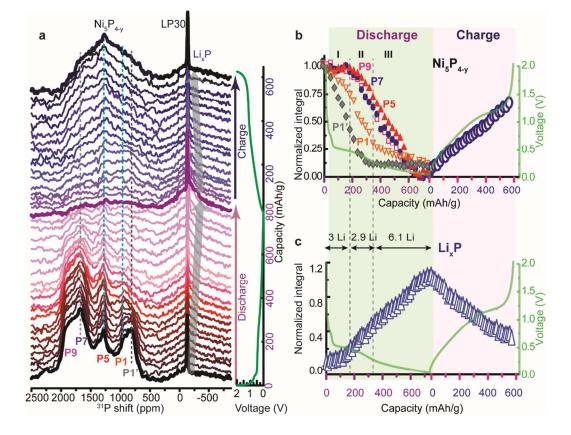
**Fig. 5** a) In operando <sup>31</sup>P NMR spectra of a Ni<sub>5</sub>P<sub>4</sub>//Li half-cell battery during the 1<sup>st</sup> cycle and the corresponding electrochemical profile. b) and c) Normalized area integrals of <sup>31</sup>P NMR resonances from Ni<sub>5</sub>P<sub>4-y</sub> and Li<sub>x</sub>P, respectively.
