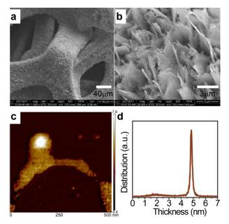
**Fig. 1** Microscopic images of the *in situ* synthesized Ni<sub>5</sub>P<sub>4</sub> nanosheets supported on Ni foam. (a) and (b) are SEM images with different magnifications of the nickel phosphide on Ni foam, (c) the AFM image, and (d) the histogram of nanosheet thickness obtained from the analysis of AFM results.
