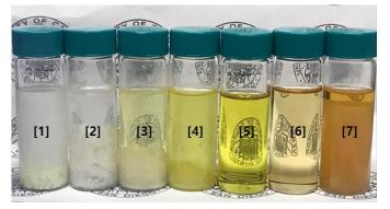
**Fig. 1.** Images of THF solutions dissolving  $P_2S_5$  and  $LiSC_2H_5$  with different molar ratios of 1:0, 1:0.1, 1:0.3, 1:0.5, 1:1, 1:3, and 1:6 from [1] to [7], respectively. 10 g of THF solvent is used in each solution.
