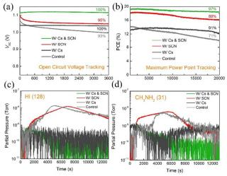
**Fig. 6.** (a) Open-circuit voltage and (b) MPP tracking of  $V_{OC}$  of PVSCs without encapsulation under a 100 mW/cm<sup>2</sup> AM 1.5G illumination in ambient air. Mass spectroscopy traces for (c) HI (m/z = 128) and (d) CH<sub>3</sub>NH<sub>2</sub> (m/z = 31) released from perovskite films under light induced decomposition measurements.
