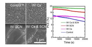
The combination of Pb(SCN)<sub>2</sub> and CsPbI<sub>3</sub> results in high quality perovskite films, leading to high performance PVSCs with stable power output.
