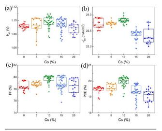
Fig. 4 Statistical results of 135 PVSCs based (MA $_{0.7}FA_{0.3})_{1\times x}Cs_xPbI_3$  perovskites with Cs content changing from 0 to 20%.
