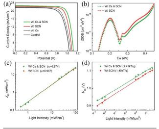
**Fig. 2** Characterizations of photovoltaic performance of PVSCs. (a) *J*-*V* curves under reverse scan of PVSCs without and with Cs and/or SCN. (b) Trap density of states and light density dependence of (c)  $J_{SC}$  and (d)  $V_{OC}$  of W/ SCN and W/ Cs & SCN.
