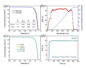
**Fig. 5** Photovoltaic parameters of the best-performing PVSCs with 10% Cs. (a) *J-V* curves measured under reverse and forward voltage scans with a scan rate of 1V/s. (b) The EQE plot and integrated current density curve. (c) *J-V* curves measured under reverse voltage scan with different scan speeds. (d) MPPT profile of the best-performing PVSC under 100 mW/cm<sup>2</sup> AM 1.5G illumination.
