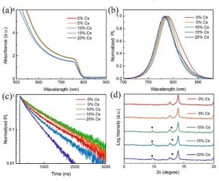
Fig. 3 (a) Absorbance, (b) Normalized PL, (c) PL decay and (d) XRD patterns of Pb(SCN)<sub>2</sub>-incorporated ( $MA_{0.7}FA_{0.3}$ )<sub>1×</sub>Cs<sub>x</sub>Pbl<sub>3</sub> films with x varying from 0 to 20%. This journal is © The Royal Society of Chemistry 20xx
