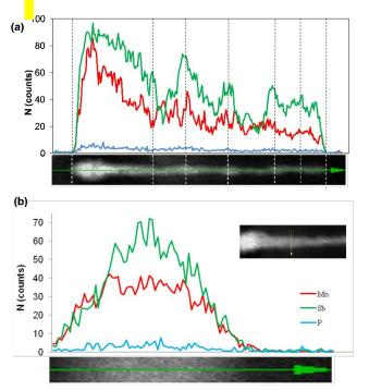
**Figure 6:** HAADF-STEM of a MnSb nanoparticle with a 'swollen tail' synthesized in the presence of 2.64 mmol of NaBH<sub>4</sub> and line scan elemental analysis (a) axial (b) vertical scan across the tail: Sb (green) Mn (red) and P (cyan).
