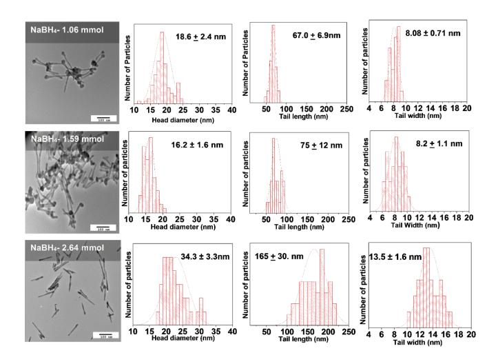
**Figure 4**: TEM images of MnSb syntheses in the presence of different amounts of  $NaBH_4$  (1.06-2.64 mmol) and associated histograms corrosponding to the head diameter, tail length, and tail width
