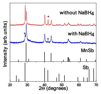
**Figure 1:** PXRD data of the product of MnSb synthesis carried out in the absence and in the presence of NaBH<sub>4</sub> (0.53 mmol). The corresponding peaks for Sb, (012) at  $2\Theta$ =28.7 and (110) at  $2\Theta$ =42, are marked with asterisks for comparison. (MnSb-PDF # 03-065-0388, Sb-PDF # 00-035-0732)
