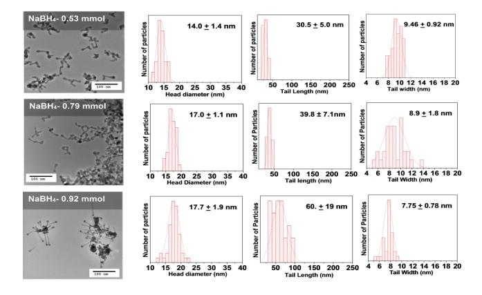
**Figure 3**: TEM images of MnSb syntheses in the presence of different amounts of  $NaBH_4$  (0.53-0.92 mmol) and associated histograms corrosponding to the head diameter, tail length, and tail width.
