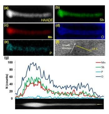
Figure 5: (a) HAADF-STEM of MnSb nanoparticles synthesized in the presence of NaBH<sub>4</sub> (2.64 mmol) and EDS mapping of (b) Sb and (c) Mn (d) O and (e) P; (f) Bottom mount image of a portion of the tail part of a MnSb nanoparticle showing lattice fringes; (g) line scan elemental analysis of a single head-tail MnSb nanoparticle: :Sb (green), Mn (red), O (blue), and P (cyan).
