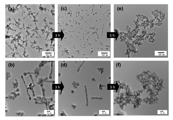
**Figure 8:** Low and high magnification TEM images showing the transformation of initial elongated head-tail nanorods, [(a) (low mag), (b) (high mag)] into mixed head-tail nanorod and spherical nanoparticles 3h after adding 0.9 mmol of  $Mn_2(CO)_{10}$  [(c) (low mag), (d) (high mag)] and into spherical nanoparticles after 5 h total [(e) (low mag), (f) (high mag)].
