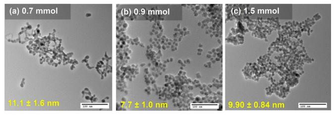
**Figure 7 (a-c):** TEM images of MnSb nanoparticles synthesized in the presence of NaBH<sub>4</sub> (0.79 mmol), using 0.7, 0.9, 1.5 mmol (40, 80, 200% mole excess) of  $Mn_2(CO)_{10}$  (particle diameter refers to the head diameter).
