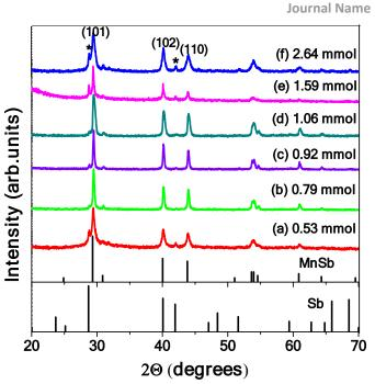
**Figure 2:** PXRD data of the product of MnSb synthesis (1 mmol Sb and 1.2 mmol Mn) as a function of added NaBH<sub>4</sub>. The asterix denotes the position of elemental Sb; the principal peaks of MnSb are labeled. (MnSb-PDF # 03-065-0388, Sb-PDF # 00-035-0732).
