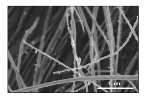
**Figure 2**:High-resolution SEM image showing conversion of carbon nanofibers of different diameters, where thin fibers are completely converted into diamond and thick fibers show diamond formation on the surface. Some of the surface nuclei grow into nanodiamond rods normal to the substrate along the diameter.
