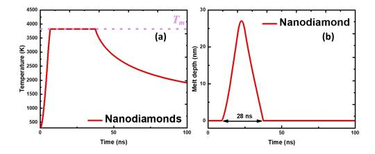
**Figure 6**: SLIM calculations using the following parameters: Melting temperature: 3823 K, Evaporation temperature: 5000 K, Latent heat of melting: 19775 J/cm3, Thermal conductivity of
