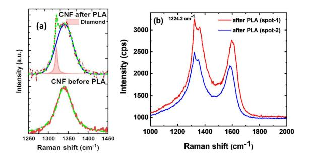
**Figure 4**: (a) Raman spectra before and after laser annealing in CNF, clearly showing diamond peak near 1321cm<sup>-1</sup>, which downshifted from standard 1332 cm<sup>-1</sup> peak as result of phonon confinement, and (b) Raman spectra after PLA in CNT showing the sharp diamond peak at 1324.2 cm<sup>-1</sup>.
