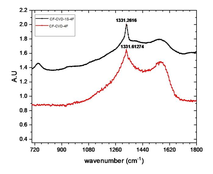
**Figure 11**: Characteristic Raman spectra from HFCVD grown diamond on treated and untreated carbon fibers, showing some graphitic peak in untreated samples.
