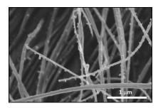
We report a pulsed laser annealing method to convert carbon fibers and nanotubes into diamond fibers at ambient conditions.
