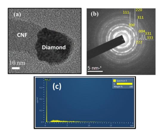
**Figure 5**: (a) TEM micrograph showing carbon nanofiber and diamond formation at the tip; (b) SAED pattern showing characteristic diamond diffraction rings, and (c) SEM-EDX of CNF after PLA.
