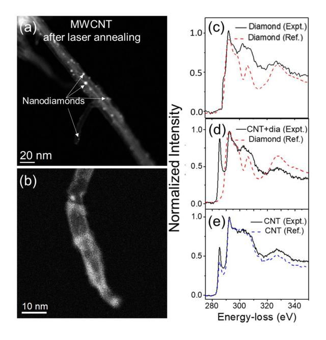
**Figure 8**: (a) HAADF image of CNTs after laser annealing showing the formation of nanodiamonds, (b) HAADF image of single CNT showing the formation of nanodiamonds at its edges and the end, EELS spectra of (c) diamond, (d) CNT and diamond obtained from the corresponding regions in laser annealed CNT, and (e) CNT before pulsed laser annealing. The reference spectra of diamond and CNT are also shown in figure (c) and (e), respectively for comparison.
