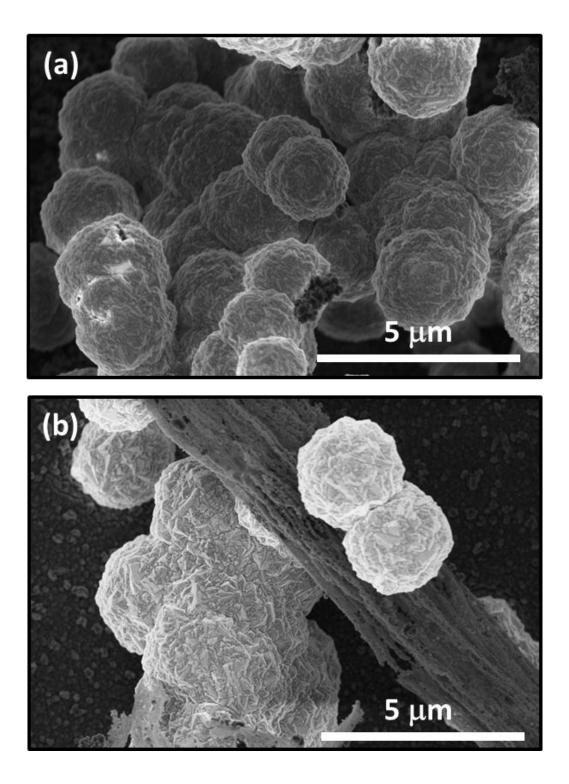
**Figure 10:** (a) Mechanism of HFCVD growth from laser treated fibers, showing multiple layers of diamond growth; and (b) Details of HFCVD growth of diamond on untreated fibers. Laser treated fibers provide much more effective sites for diamond growth during HFCVD.
