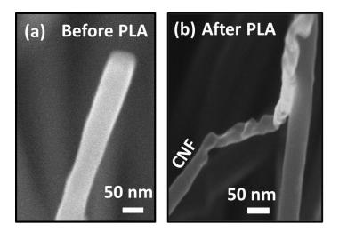
**Figure 1**: High-resolution SEM images of (a) A CNF before PLA technique, (b) CNF after PLA showing the conversion carbon nanofibers into diamond nanofibers.
