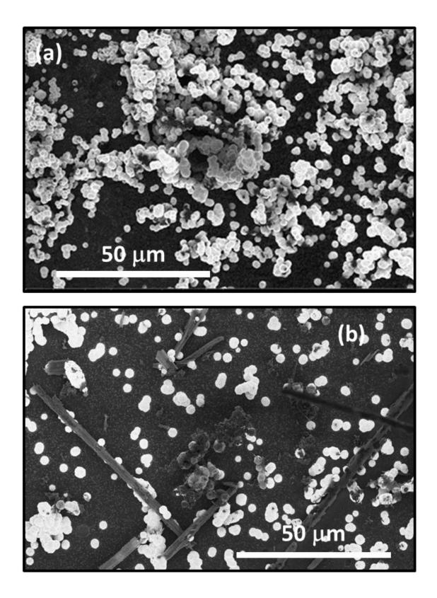
**Figure 9**: (a) HFCVD growth of diamond after laser annealing of carbon fibers (five microns diameter) with one pulse; and (b) HFCVD growth on untreated carbon fibers for a comparison.
