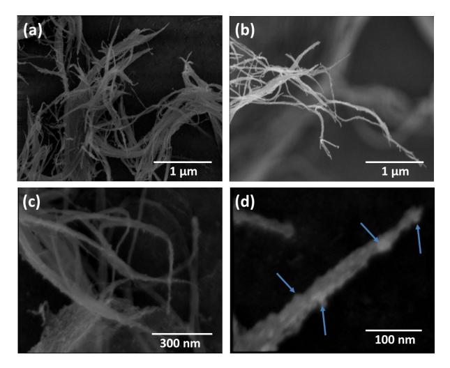
**Figure 7:** Conversion of carbon nanotubes into diamond nanorods; (a) SEM micrograph showing conversion of carbon nanotubes into diamond after 10 pulses of ArF laser (pulse duration 20ns) at 0.65 Jcm<sup>-2</sup>; (b) and (c) details of conversion process starting from the tips; and (d) nucleation of diamond in the middle of the nanotube and growth of diamond nanorods normal to the tube (shown by arrows).
