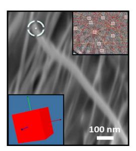
**Figure 3**: SEM micrograph of laser treated fibers with EBSD (Kikuchi) pattern characteristic of diamond and relative orientation (red cube) of diamond formed.
