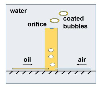
FIG. 2: Mechanism to generate oil-coated bubbles.
