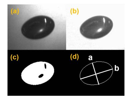
FIG. 3: Steps followed in the image processing: (a) Substract the background, (b) convert into a binary image, (c) capture the boundary of the bubbles and (d) calculate the aspect ratio.
