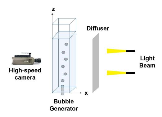
FIG. 1: Schematic diagram of the experiment apparatus.
