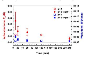
**Figure 5.** Adhesion force and work done in removing the DN hydrogel probe from the brush surface for different times after immersion in pH 1 solution for samples that were either brought into contact at pH 1 or pH 6. The applied force in both cases was 0.1 N, and was applied 2 min. The force-distance curves for these data are shown in the ESI
