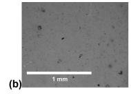
Figure 2. Optical microscope images of PDEAEMA brush layers after adhesion to the SN hydrogel (a) and the DN hydrogel (b). The scale is the same in both images and the bar represents 1 mm. Cohesive failure is clearly visible on the first brush resulted after detaching from the SN hydrogel at pH 6, whereas the DN hydrogel leaves no visible mark on the film. These images were taken after one test in DI water
