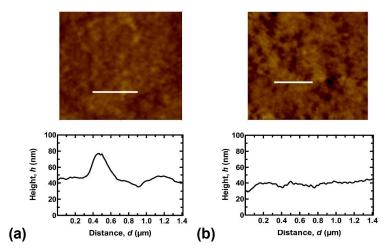
**Figure 3.** Scanning force microscopy images of the PDEAEMA brush surfaces (a) before and (b) after contact with the DN hydrogel. The surface morphology remains unaltered, but there is a small decrease in the root-mean-square roughness after the experiment from 9.8 to 5.6 nm. These images were taken after one test cycle at pH 6. The height profiles are taken from the white line on each image
