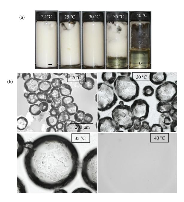
**Figure 9.** (a) Appearance of vessels containing 8 wt.% MA in HOSO before (upper) and after (lower) whipping at different temperatures, scale bar = 1 cm and (b) optical microscope images of mixtures after whipping for temperatures given, scale bar same in all cases.
