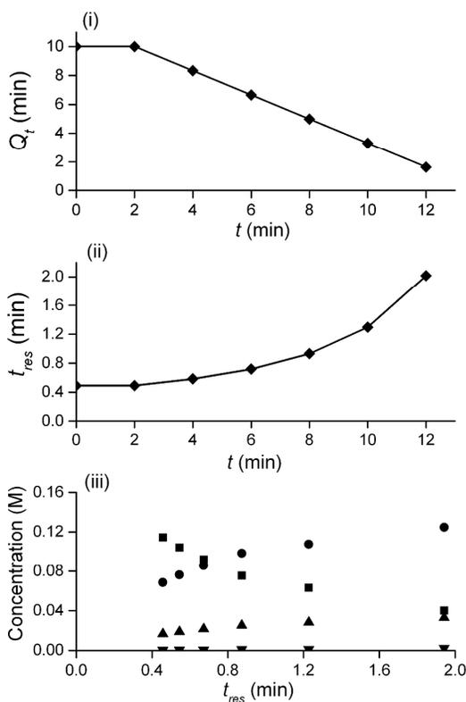
**Figure 3.** i) total volumetric flow rate ( $Q_{total}$ ) change throughout the duration of a ramp,  $\blacklozenge$  HPLC injection; (ii) residence time,  $\tau$ , as a function of operation time,  $t$ ; (iii) resulting concentration-residence time profile generated from a typical multi-step reaction scenario,  $\blacksquare$  2,4-DF 1,  $\bullet$  ortho-3,  $\blacktriangle$  para-4,  $\blacktriangledown$  bis-5.
