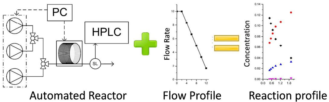
$S_NAr$  reaction profiles were generated using an automated reactor, collected in less than 3 hours, allowed accurate estimation of kinetic parameters.
