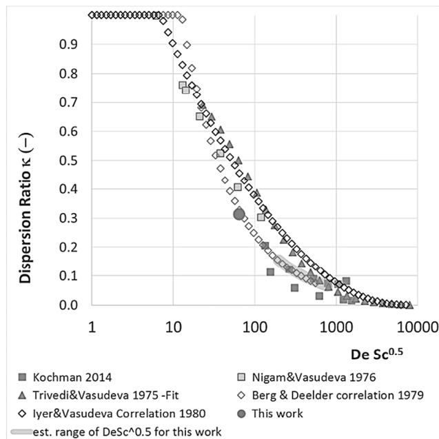
**Figure 4.** The dispersion ratio  $\kappa$  vs  $DeSc^{0.5}$  for various literature data. Where possible data have or correlations have been taken from the papers. If the data could not be retrieved and no correlation was given the data has been fitted with a line that visually represents the data well.
