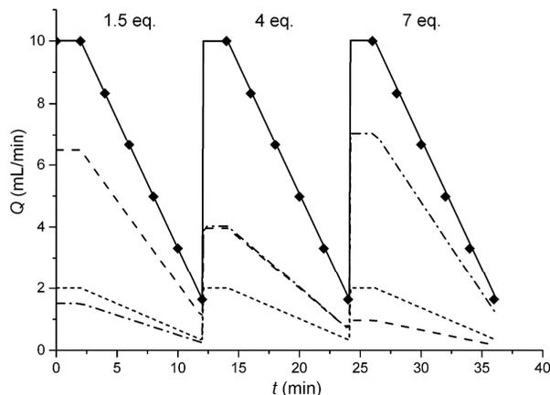
**Figure 2.** Changes in volumetric flow rate over time, where  $Q_{p1}$ ,  $Q_{p2}$ ,  $Q_{p3}$  and  $Q_{\text{total}}$  were for ..... pump 1 (Ar in EtOH), --- pump 2 (EtOH), - - - pump 3 (pyrrolidine in EtOH), — total volumetric flow rate, and ◆ HPLC injection respectively. The linear flow ramps correspond to pyrrolidine **2** to 2,4-difluoronitrobenzene **1** molar ratios: (i) 1.5:1, (ii) 4:1 and (iii) 7:1 using  $Q_{\text{total}}$  from 10 to 1.5  $\text{mL min}^{-1}$ .
