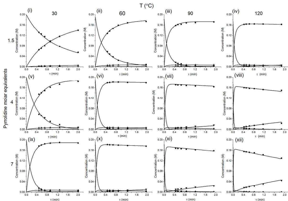
**Figure 5.** Concentration-time profiles from simultaneous parameter fitting, points = experiments ■ 2,4-DI 1, ● ortho-3, ● para-4, ▼ bis-5, lines = model using Table 1 kinetic parameter estimates.
