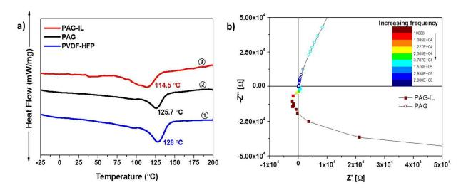
**Fig 5**. **a)** DSC thermograms of 1 PVDF-HFP 2 PAG and 3 PAG-IL. **b)** Nyquist response of the PAG and PAG-IL analyzed from 1 kHz to 10 MHz
