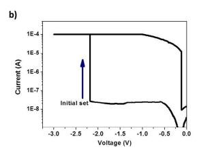
**Fig 4. a)** Initial cyclic I-V measured in the Au/PAG-IL/Au system. **b)** Zoom on the initial set process taking place at -2.2 V.
