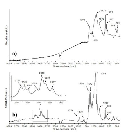
Fig 2. ATR FTIR spectra a) PAG b) PAG-IL
