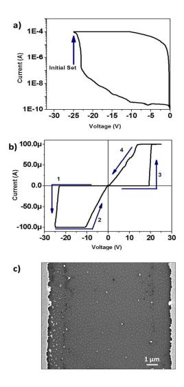
**Fig 3. a)** Initial set process, taking place at -25 V. **b)** Cyclic I-V measured in the Au/PAG/Au system **c)** FESEM image of the device with active switching matrix (AgNO<sub>3</sub> and PVDF-HFP) spin coated between the gold electrodes, after electrical characterization.
