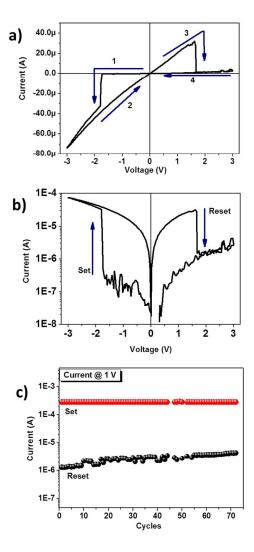
**Fig 10. a)** Cyclic I-V measured in the Au/PAG-IL/ITO system. **b)** Zoom on the set and reset process in logarithmic scale. **c)** Pulse characterization - sample was made to read at 1 V, by setting and resetting the device at -5 V and 2 V for 500 μs.
