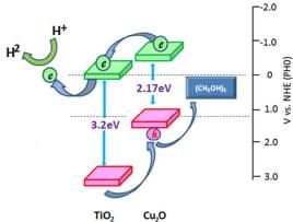
Fig. 8. (A) Photoresponse of (a)  $TiO_2$  NTAs, (b) 0.5M sample, and (c) 1.0M sample. (B) Average hydrogen yield within 10 hours. (C) Schematic of photocatalytic hydrogen evolution using  $Cu_2O/TiO_2$  NTAs as the photoanodes.
