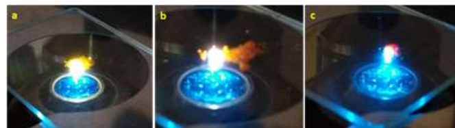
Fig.13. Phosphors ((a) FTP-, (b) DFTP-, (c) TFTP- Acetophenone under blue ray excitation.
