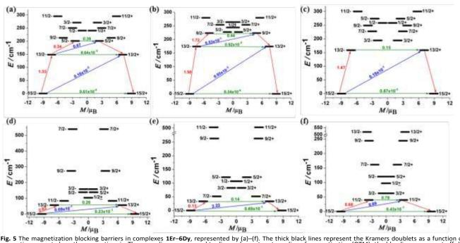
Fig. 5 The magnetization blocking barriers in complexes 1Er–6Dy, represented by (a)–(f). The thick black lines represent the Kramers doublets as a function of their magnetic moment along the magnetic axis. The green lines correspond to diagonal quantum tunneling of magnetization (QTM), the blue lines represent off-diagonal relaxation process. The numbers at each arrow stand for the mean absolute value of the corresponding matrix element of transition magnetic moment
