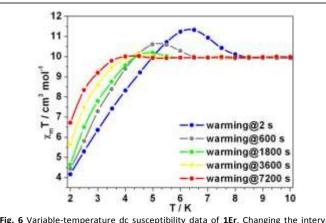
Fig. 6 Variable-temperature dc susceptibility data of 1Er. Changing the interval time can make the unexpected rising disappear.
