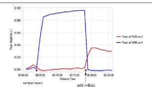
**Fig. 2** In situ IR plot of the lithiation of **3** with *n*-BuLi in THF at -50 °C with time in h:min:sec.  $v_{c=0}$  **3** 1696 cm<sup>-1</sup>, *n*-BuLi added at time 18 min,  $v_{c=0}$  lithiated **3** 1636 cm<sup>-1</sup>.
