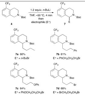
Scheme 2 Lithiation–substitution of the tetrahydroisoquinoline 4.
