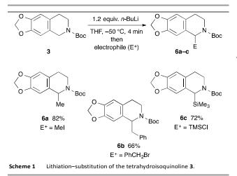
By using the optimised lithiation conditions (THF, -50 °C, 4 min), followed by electrophilic quench and purification by column chromatography, the substituted products **6a–c** were obtained with reasonable to good yields (Scheme 1). Lithiation occurs only in the benzylic position, as judged by <sup>1</sup>H NMR spectroscopy. We did not observe any other substitution products.
