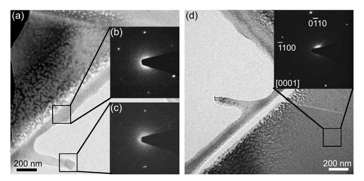
Fig. 3 (a)TEM image of a hBN flake that contains an etch pit (bottom right-hand corner) fabricated by EBIE. The insets (b) and (c) show selected area electron diffraction patterns from the regions indicated on the image. The region indicated in (d) shows a pristine area of the hBN flake and the inset shows its corresponding selected area electron diffraction pattern. All patterns were indexed as hBN.
