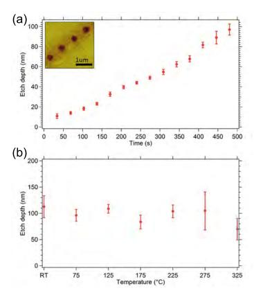
**Fig. 5** (a) Etch pit depth plotted as a function of etch time at room temperature. The inset is an AFM image of some of the etch pits used to make the plot. (b) Etch pit depth of hBN versus temperature. The electron beam dwell time was 10 minutes at each temperature.
