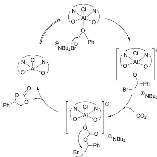
**Scheme 4** Proposed reaction mechanism for the cycloaddition of epoxides into CO<sub>2</sub> with catalyst system **1**/TBAB.
