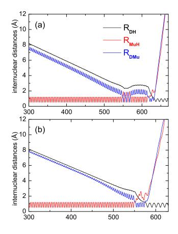
FIG. 5: Plot of internuclear distances as a function of time for two trajectories (a) and (b) leading to DH formation below the vibrationally adiabatic collinear barrier. As can be seen, a shortlived collision complex is formed allowing the formation of DH in spite of an initial D-Mu–H configuration.
