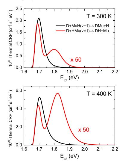
FIG. 6: Thermal cumulative reaction probabilities,  $C_R(E_{\text{tot}};T)$ , for the two exit channels of the D+HMu(v=1) reaction. Upper panel: T=300 K. Lower panel: T=400 K. Please, note that the curve for DH formation has been multiplied by 50.
