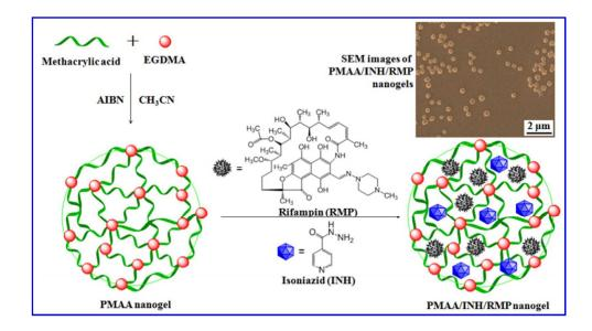
**Figure 8.** Preparation of the PMAA/INH/RMP nanogel: Step 1, Methacrylic acid, EGDMA, and AIBN were added into CH3CN to obtain a PMAA nanogel; Step 2, Isoniazid (INH) and Rifampin (RMP) were loaded into the PMAA nanogel to produce the PMAA/INH/RMP nanogel. (Inset: SEM images of the obtained PMAA/INH/RMP nanogels.) Reprinted with permission from Reference<sup>129</sup> Copyright (2016), with permission from Elsevier.
