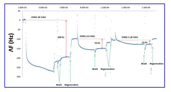
**Figure 9.** Frequency shifts (DF) corresponding to different titres of AIVH5N1 (64, 6.4 and 1.28 HAU, respectively) for aptamer hydrogel I coated QCM sensor. Reprinted from Reference <sup>146</sup> Copyright (2016), with permission from Elsevier.
