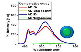
**Fig. 8** Photoluminescence spectra of bi-polymer NPs (ADN3) prepared through click reaction and ADBr prepared from non-functionalized polymers.  $\lambda_{ex}$ =350 nm (red and blue lines) and 444 nm (dark and light green lines).
