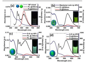
Fig. 5 Absorbance and emission spectra of bipolymer NP dispersion in water (a) NP Mixed (PFB-N3+PFBT-P NPs) (b) Soln NP (mixing the two polymers solutions prior to NP formation) (c) DA 45 NP (PFB-N3/PFBT-P) (d) AD 45 NP (PFBT-P/PFB-N3) ( $\lambda_{ex}$ =350 nm)
