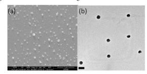
Fig. 10 Size and morphology of DAR 4% NPs  ${\sim}101nm$  (a) SEM micrograph (scale 1µm) and (b) TEM micrograph (scale 0.2 µm)
