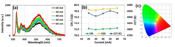
Fig. 13(a) The spectra and (b) CRI, CQS, and CCT of the tandem nanoparticle integrated white LED at varying current levels and (c) corresponding CIE coordinates.
