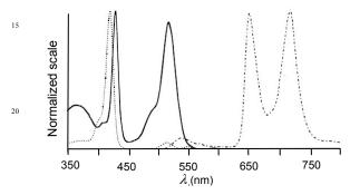
25 Fig. 4 Overlay of the absorption spectrum of FbTPP (dashed line. Fb = free base) with the absorption spectrum (solid line) and the fluorescence emission spectrum (dot-dashed line) of 17 obtained upon illumination at 485 nm (toluene, 298 K). Reproduced with permission from Li et al.<sup>66</sup>
