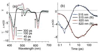
**Fig. 8** (a) Ultrafast transient absorption spectra of **22** after excitation at <sup>40</sup> 508 nm (10–300 ps). (b) Transient absorptions at 515 nm (BODIPY) and 620 nm (porphyrin) with predicted traces based on kinetic parameters for the system. Reproduced with permission from Whited et al.<sup>65</sup>
