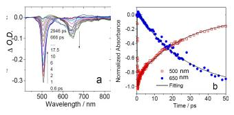
Fig. 41 Picosecond ultrafast transient absorption spectra of 67 upon <sup>35</sup> femtosecond pulsed laser excitation at 504 nm. (a) Transient absorption spectra after pulsed laser excitation at 504 nm. (b) Decay traces at 500 nm and 650 nm.  $c = 1.0 \times 10^{-5}$  M in toluene at 20 °C.<sup>64</sup>
