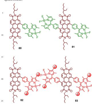
Fig. 48 Broadband visible light-harvesting PBI-Bodipy dyad 82 and triad 83 with competing ISC and FRET process. Dyad 80 and triad 81 were prepared as reference compounds.<sup>102</sup>
