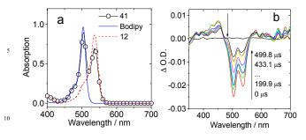
Fig. 22 (a) The UV-vis absorption of 41 and the energy donor and energy acceptor reference compounds (12 and Bodipy), in toluene,  $c = 1.0 \times 10^{-5}$  M. (b) The nanosecond transient absorption of 41 in deaerated toluene,  $\lambda_{ex}$  15 = 532 nm,  $c = 1.0 \times 10^{-6}$  M, 20 °C.<sup>56</sup>
