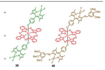
Fig. 20 Broadband visible light-absorbing subphthalocyanine triads 39 and  $40.^{\rm 104,105}$
