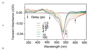
**Fig. 11** Femtosecond transient absorption spectra for **26** obtained with a 530 nm pump pulse. The 530 nm excitation directly excites the  ${}^{1}\pi\pi^{*}$  absorption band of the Bodipy moiety. Reproduced with permission from Lazarides et al.<sup>86</sup>
