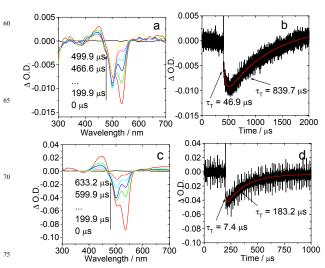
**Fig. 23** Intermolecular triplet-triplet-energy-transfer (TTET) observed with nanosecond transient absorption spectra. (a) *c* [Bodipy] =  $5.0 \times 10^{-6}$  mol/L, *c* [bodipy] : *c*[**12**] = 5:1, (b) The decay trace at 500 nm, (c) *c* [Bodipy] =  $1.0 \times 10^{-5}$  mol/L, *c* [Bodipy]: *c* [**12**] = 1:1. (d) The decay trace so at 500 nm,  $\lambda_{ex} = 535$  nm. In Toluene. 20 °C.
