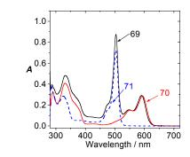
Fig. 43 UV-vis absorption of Pt(II) complexes.  $c = 1.0 \times 10^{-5}$  M, in toluene at 20 °C.<sup>132</sup>
