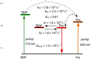
Fig. 9 Jablonski diagram summarizing the excited-state behaviour of complex 22 upon selective photoexcitation into the BODIPY or
