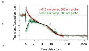
Fig. 12 Kinetics of 26 at probe wavelengths of 500 and 489 nm, following excitation at 530 (green symbols) or 600 or 615 nm (red symbols). The kinetics at these probe wavelength are indicative of the bleach of the Bodipy  $\pi\pi^*$  absorption band. Reproduced with permission <sup>55</sup> from Lazarides et al.<sup>86</sup>
