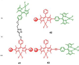
**Fig. 21** Bodipy-diodoBodipy dyads as triplet photosensitizers **(41, 42, 43)** (Bodipy moiety is the energy donor, iodoBodipy moiety is the energy <sup>105</sup> acceptor and the spin converter).<sup>56</sup>
