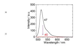
Fig. 26 Fluorescence emission spectra of 47 and the triplet <sup>40</sup> photosensitizer 45,  $\lambda_{ex} = 490$  nm.  $c = 1.0 \times 10^{-5}$  M in toluene 20 °C.<sup>58</sup>
