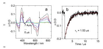
**Fig. 31** (a) Nanosecond transient absorption spectra of **48** ( $\lambda_{ex} = 532$  nm). (b) Decay curve of **48** at 630 nm,  $c = 1.0 \times 10^{-5}$  M, in deaerated CH<sub>2</sub>Cl<sub>2</sub>. 20 °C.<sup>57</sup>
