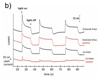
Fig. 8. a) Schematic of the EPI photoconductor sample showing the SUB-anchored RC on the surface of the EPI crystallites. The aqueous solution is maintained over the active area of the device with the help of a PDMS block. b) Current transients obtained for the EPI photoconductor devices with bias voltage of 0.5V. A  $\approx$ 50 nA dark-current characterized all devices.
