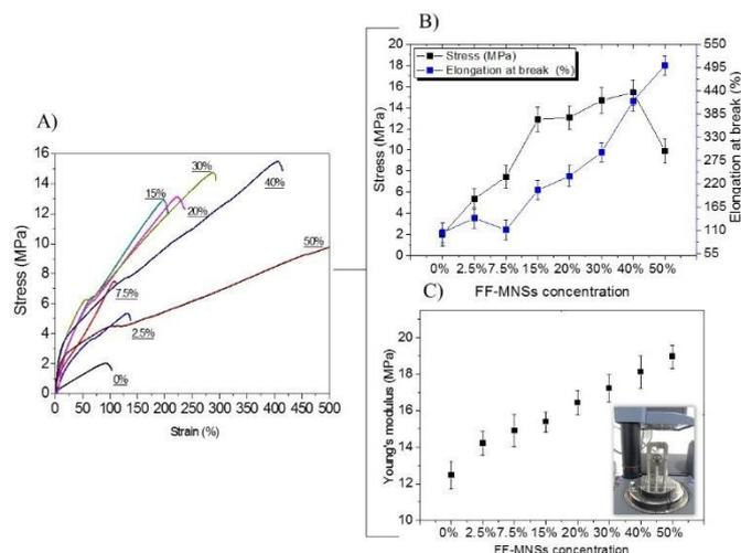
**Figure 3.** (A) Stress–strain curves from electrospun samples; (B) Stress and elongation at break behaviour upon peptide concentrations in the formulations; (C) Young modulus for the different peptide concentrations.
