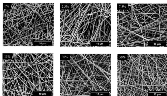
**Figure 1.** Scanning electron micrographs from polymeric electrospun membranes at different FF/PCL percentages.
