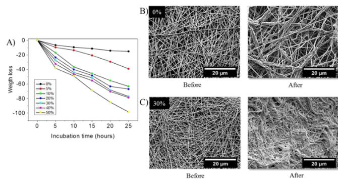
**Figure 6.** (A) Percentage weight loss for PCL and PCL-FFMNTs composites after 25 hours incubation; (B-C) FEG-SEM of PCL and the 30% FF-MNT sample before and after enzymatic incubation. The biodegradation occurs from the surface to the inside of the fiber.
