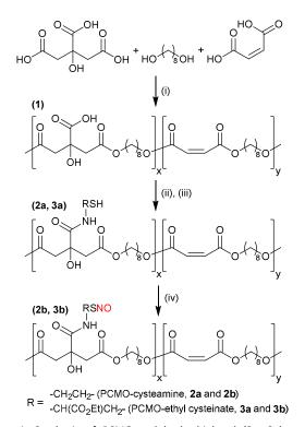
**Figure 1.** Synthesis of PCMO and both thiolated (2a, 3a) and *S*nitrosated (2b, 3b) derivatives. (i) 140 °C, 2 h, (ii) NHS, EDC·HCl, 0 °C to RT, overnight, cysteamine hydrochloride/ethyl cysteinate hydrochloride, RT, 48 h, (iii) DTT, TEA, RT, 1 h, (iv) *t*-BuONO, EtOH, RT, 4h.
