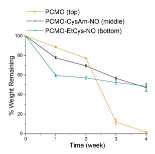
Figure 3. Degradation profiles of PCMO and S-nitrosated derivatives under physiological conditions (pH 7.4 PBS, 37 °C).
