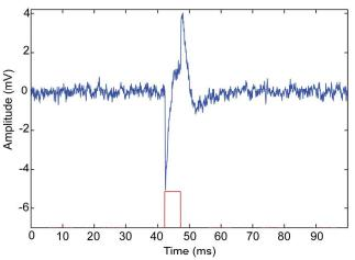
**Figure 6:** Photoelectric Artifact with a 473 nm laser set to 10mW. Red indicates 5 ms wide laser pulse onto a photosensitive 10  $\Omega$ -cm boron-doped silicon substrate. Ionic currents (blue) were recorded 100 μm away in 0.5% agarose in PBS. Note: the lead electrical artifact is negative and a positive deflection occurs after the laser pulse ends. †††
