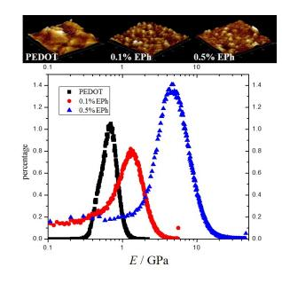
Figure 8 AFM QNM modulus distribution. (a) AFM image of the polymer films (2  $\mu$ m by 2  $\mu$ m); (b) AFM QNM modulus distribution of PEDOT, 0.1% EPh and 0.5% EPh
