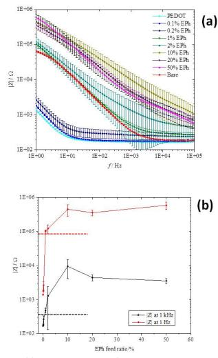
**Figure 7** (a) Impedance amplitude of PEDOT and PEDOT-co-EPh copolymers as a function of frequency; (b) impedance amplitude at 1 Hz and 1 kHz for the PEDOT-co-EPh copolymers as a function of EPh content; dashed lines indicate the impedance amplitude of bare Pt electrode at 1 Hz (red) and 1 kHz (black), respectively. (Deposition charge: 288 mC/cm<sup>2</sup>)
