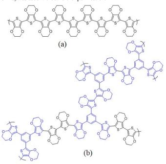
Figure 1 (a) PEDOT and (b) EPh crosslinked PEDOT.
