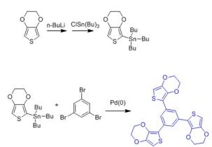
Scheme 1 Synthesis route of 1,3,5-Tri[2-(3,4-ethylenedioxythienyl)]benzene (EPh)
