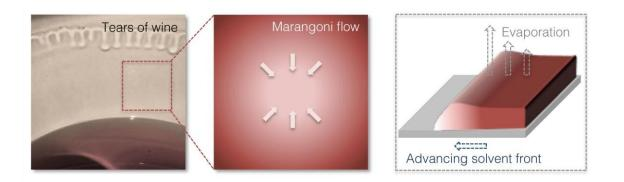
**Figure 1.** Representative photograph shows the uniform coating of red wine at macroscale enabled by the Marangoni flow. The dissimilar evaporation rates between each solvent result in advancing solvent fronts toward un-wetted areas.
