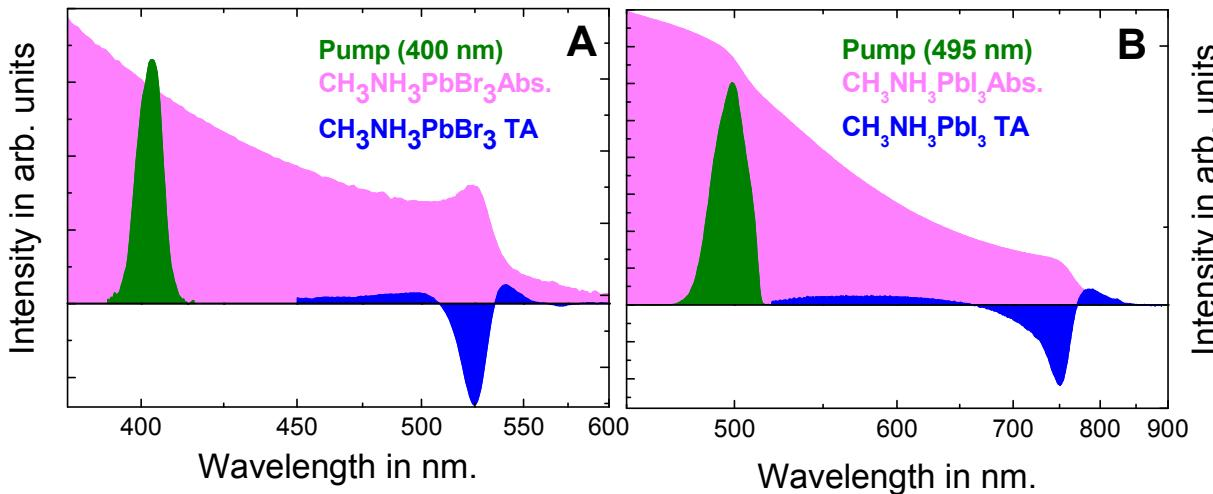
**Figure 1:** Spectroscopic details of the experiments, including steady state absorption spectra of both samples, along with the pump pulses used to excite them, and TA spectra obtained at a pump-probe delay of 250 fsec.
