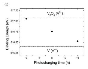
Figure 7 (a) XPS spectra for BiVO4 photoanodes photocharged for 0 (black), 8 (red) and 16 h (blue) in K-Pi buffer pH 7.2. (b) V2p3/2 peak position for BiVO4 samples photocharged for different amount of time. V2O5 and V(IV) binding energies are shown for reference.
