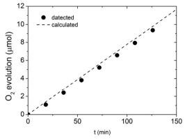
Figure 8 Gas chromatography detection of  $O_2$  evolved at photocharged BiVO<sub>4</sub> electrode at constant current of 0.65 mAcm<sup>-2</sup>.
