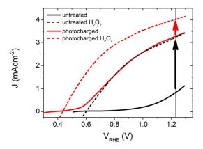
Figure 1 J-V scans of 200 nm thick  $BiVO_4$  under back-side AM1.5 illumination, in 0.1 M K-P<sub>i</sub> buffer (pH 7.2), scan rate 50 mVs<sup>-1</sup>, anodic sweeps. Arrows denote catalytic limitations for untreated (black) and photocharged (red) material.
