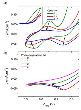
Figure 6 JV scans under illumination, for (a) untreated BiVO4, inset: full potential range, and (b) BiVO4 photocharged for different periods of time (cathodic sweeps only).
