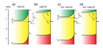
Figure 3 Estimated electronic band diagrams for BiVO4 in the OC configuration without surface states present (a) in the dark and (b) under illumination, and with surface states present (c) in the dark, and (d) under illumination.
