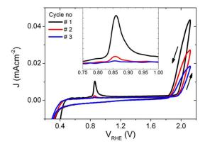
Figure 5 The first three dark JV scans of the BiVO4 photoanode after 10 hours of photocharging, inset: a zoomed in plot around the observed oxidation peak at  $^{\sim}0.85$  VRHF.
