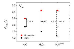
Figure 4 Equilibrium potentials and photovoltage values of  $BiVO_4$  photoanodes in the open circuit configuration: untreated sample in 0.1M K-P<sub>1</sub> electrolyte ( $H_2O$ ), in presence of a hole scavenger ( $H_2O_2$ ), photocharged sample ( $H_2O^{photo}$ ).
