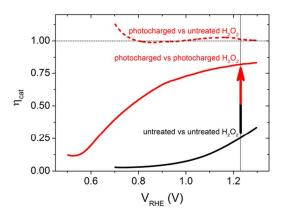
Figure 2 Calculated catalytic efficiency for the untreated (black solid curve) and photocharged BiVO<sub>4</sub> samples (red curves). The catalytic efficiency for the photocharged samples was estimated using the JV characteristics in the presence of  $H_2O_2$  for the untreated sample (dashed red curve) and with the photocharged sample (solid red curve).
