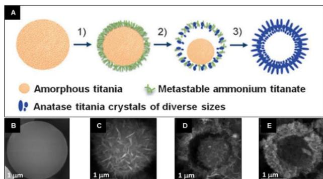
**Figure 8.** Formation of  $\text{TiO}_2$  hollow spheres by Ostwald ripening; A). Formation of  $\text{TiO}_2$  hollow spheres from amorphous titania; B,C,D,E) SEM images of each step.<sup>62</sup>
